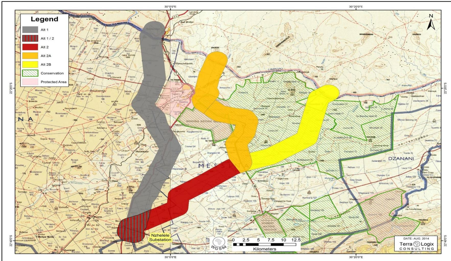
Figure 10: Distribution of the final route alternatives, with the preferred alternative being alternative 1 (grey colour) (Source: Baagi EC, March 2016)
